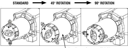
Note: Motor casing rotates with End Cap
