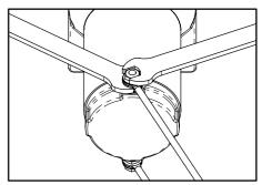
Proper Terminal Tightening
