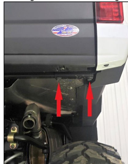
Figure 4: Factory Bolts for Removal
