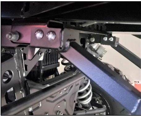
Figure 6: Lower Brackets to Machine
