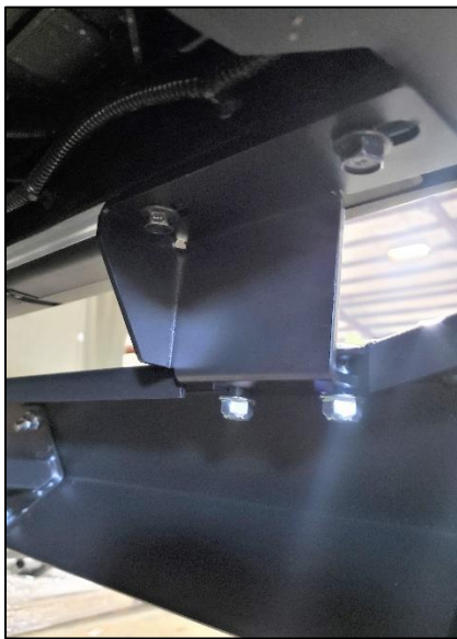
Figure 7: Upper Bracket to Machine and Bumper
