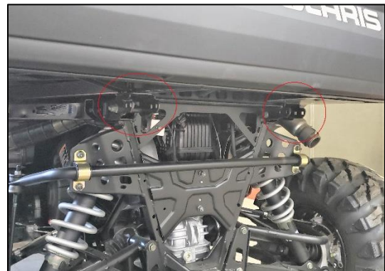
Figure 5: Lower Bracket Mounting Location
