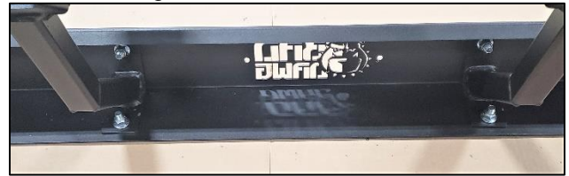
Figure 3: Upper Brackets to Bumper
