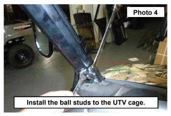
Install the ball studs and nuts to the windshield using a 16mm and 13mm socket/wrench. See Photo 5 and Photo 6.
