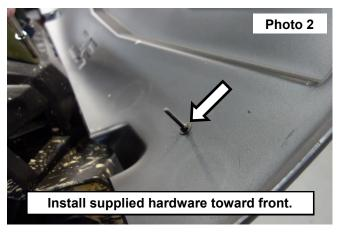
NOTE: This nut will be used as a spacer--another nut will be used to secure the roof to the UTV.
