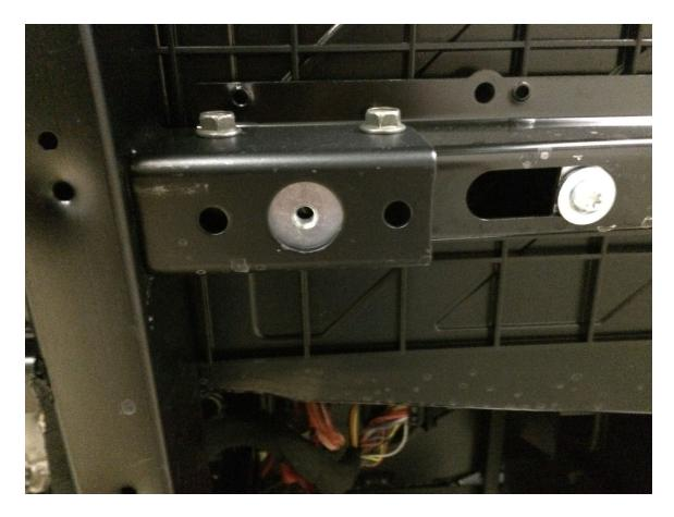
Step Thirteen: Set the floorboard skid into position and start your bolts into the bar clamp and nut plate you just installed. Use anti seize on all of these bolts, and leave loose for now.
