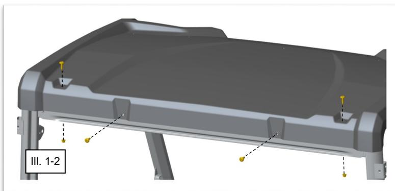
4. Loosely install three M6 x 25mm Torx Screws (Item #2) and Lock Nuts (Item #4) in the mounting holes towards the center of the Roof. Be sure not to cross thread fasteners. (See Illustration 1-3).
