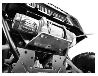
Bolt the winch in place using the hardware provided with your winch.
