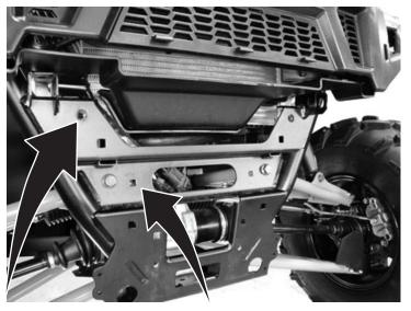
Mount will install in the top threaded holes and middle square holes with spacers in between.
