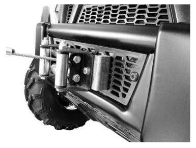
Use the roller fairlead brackets if installing a standard size fairlead or hawse.
