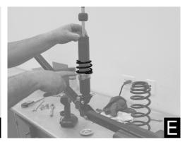
**Step 8:** Slide the Lift Spacer onto the shock (Figure F).
