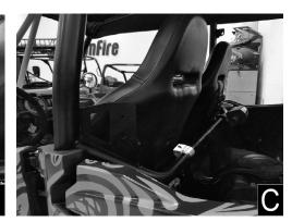
Step 5: Obtain Eyelet bolt [P3], washer [P5], and locknut [P6]. Place Eyelet Bolt [P3] through hole in bracket and then install with hardware (Figure D).
