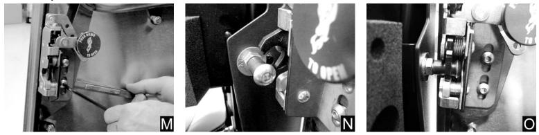
Step 25: Keeping the door closed, tighten the hardware on the latch to 6 ft-lbs (72 in-lbs).
