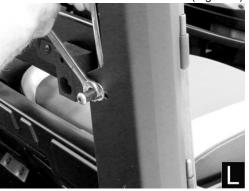
Step 20: Place one brass washer (supplied) on each hinge pin.
