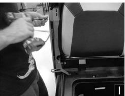
Step 9: Flip rear seat base up and remove Torx head screw similar to Figure F.
