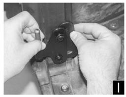
**Step 11:** Align the upper slot of the Upper Hinge Bracket - Driver [P5] to the upper hole and then loosely install the self-tapping screw [P12] with washer [P11]. Make sure to leave 1/2" gap. When done, repeat Step 9 process for the bottom slot (Figure J).
