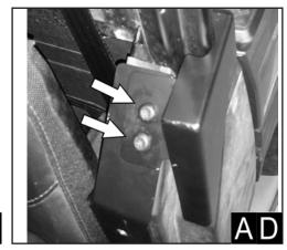
Step 31: Obtain Upper Hinge Bracket - Driver Side (threaded) [P22] and check part with image to ensure the part is correct before installing. Starting with the bottom hole, loosely install with one M8 Button Head Cap Screw [P30] and one M8 washer [P29]. Repeat for top hole.
