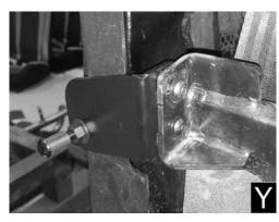
**Step 26:** Locate 2 lower factory bolts behind seat near lower seat belt attachment point (Figure Z). Remove inner bolt and retain for later use. Loosen outer bolt approximately 1/2" (Figure AA)
