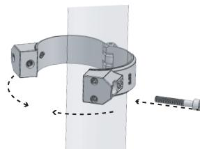
Open clamp and place around roll cage tube. Close clamp around roll cage tube, put the m5 x 30mm bolt through the hole.
