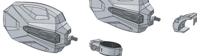
Detach clamp assembly from mirror housing assembly by unscrewing.
