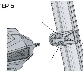
Remove mirror housing from the clamp. Tighten all clamp bolts
