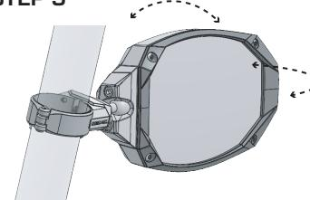
Rotate mirror on clamp so that it is level and provides desired viewing angle.
