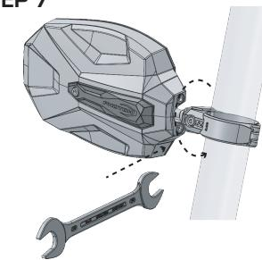
Assemble the mirror housing back onto the clamp. Use a 12mm wrench to tighten the ball stud on the clamp
