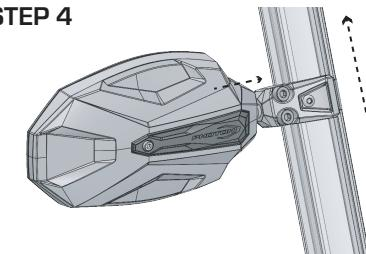
Temporarily assemble the mirror housing on the clamp to position the clamp at desired height.
