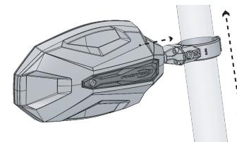
Temporarily assemble the mirror housing on the clamp to position the clamp at desired height.
