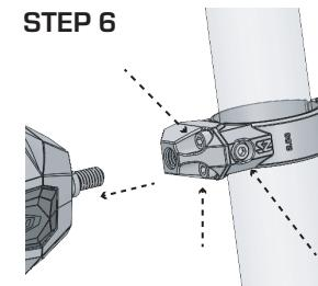
Remove mirror housing from the clamp. Tighten all clamp bolts to secure the clamp on the roll cage.
