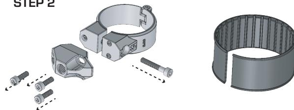
Disassemble clamp by unscrewing 4 bolts.
