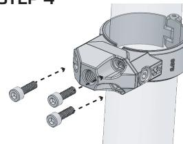
Complete the clamp assembly by putting 3 m5x16mm bolts. **DO NOT TIGHTEN THEM ALL THE WAY YET.**
