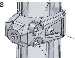
Place both halves of the clamp around roll cage tube. Complete the clamp assembly by tightening bolts. **DO NOT TIGHTEN THEM ALL THE WAY YET.**
