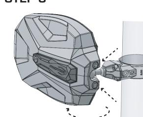
Turn the mirror housing to tighten the ball joint.
