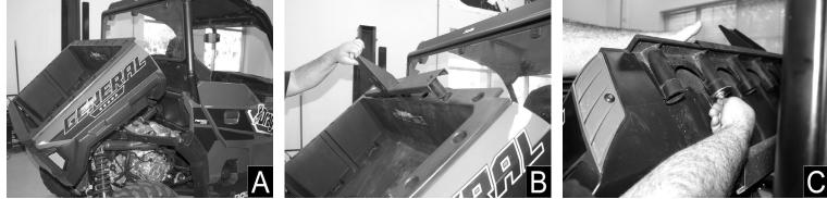
Step 5: Tighten the hardware until the part is fully secured. Ensure the hardware is not too tight that it is flexing the plastic. (Figure D) Then install P8 into the holes of the base mount.
