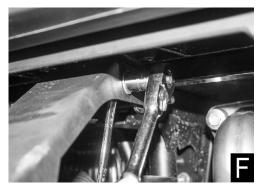
**Step 8:** Torque factory bolts from Step 6 to factory specifications. Tighten the long factory bolts until snug and then loosen until the bed is easy to pivot.
