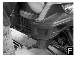
**Step 8:** Locate Bumper Cover (P2) and place on to Sub-Structure (P1) installed in previous step. (**Figure G**) Loosely install one supplied bolt (P5) into one of the top holes to hold the cover in place.
